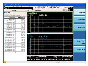
Automatically downloaded ENR data table in the NFA noise figure analyzers, X-Series Signal Analyzers and ESA E-Series spectrum analyzers with noise figure capability
