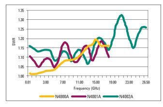
Figure 1. Characteristic SWR at 23°C
